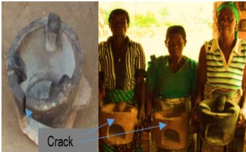
Photo 6.1: Stoves with a crack on the upper door of the stove from Chapita Village in Balaka district, and Mvuduma Village in Mulanje district (Chisoni, August 2014)
