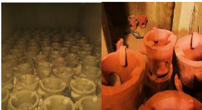
Photo 7.5: Newly produced Chitetezo Mbaula, before firing (left), after firing (right) (Chisoni June 2016b)
