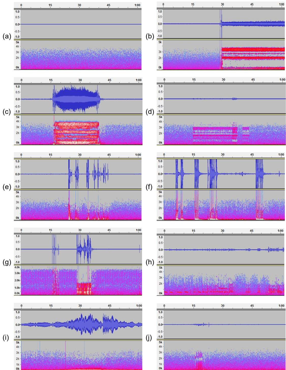
Figure 3.2 Waveforms and spectrograms of (a) white noise section with no sound recorded, (b) water running through a hosepipe, (c) water run into a bucket, (d) an indoor water use event, (e) object hitting tap and nearby objects, (f) hammering near the tap, (g) object sled over the ground near the tap, (h) dogs barking, (i) heavy vehicle passing through a nearby road and (j) mobile phone interference.
