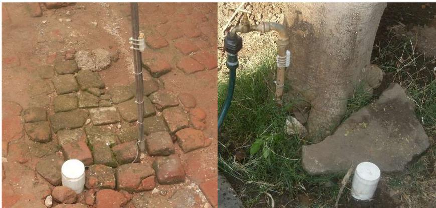
Figure 3.1 Complete setup of recorder (in PVC casing) and microphone (covered by a block of PVC rubber) at the outdoor tap.
